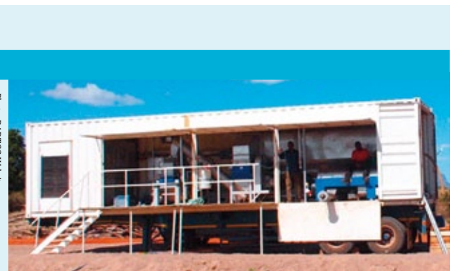
Autonomous Processing Unit (AMPU) , which prevents the spoilage of cassava, bringing the "factory to the field".
