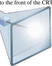
**Step 6.** An image is displayed on the screen when the electrons hit phosphor dots on the back of the screen.
