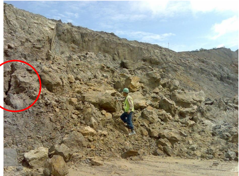
Individual slope mudstone failure on 22 Maret 2010 in Lowwall PIT RA , Height of slope = 12 m , \alpha = 48^\circ Some boulder exists between failures .
