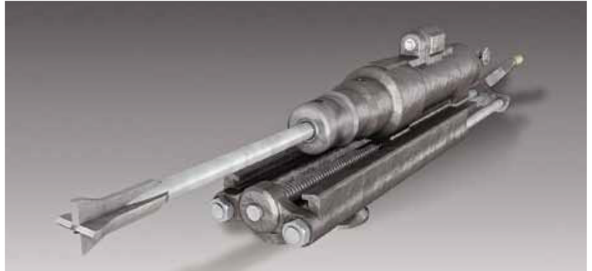
The first drill made by Atlas "pneumatic rock drill No. 16" had a weight of 280 kg (617 lb) and was heavy and difficult to handle - at least two men were needed to move it.
